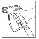
**Step 5** Press trigger to release water pressure.
